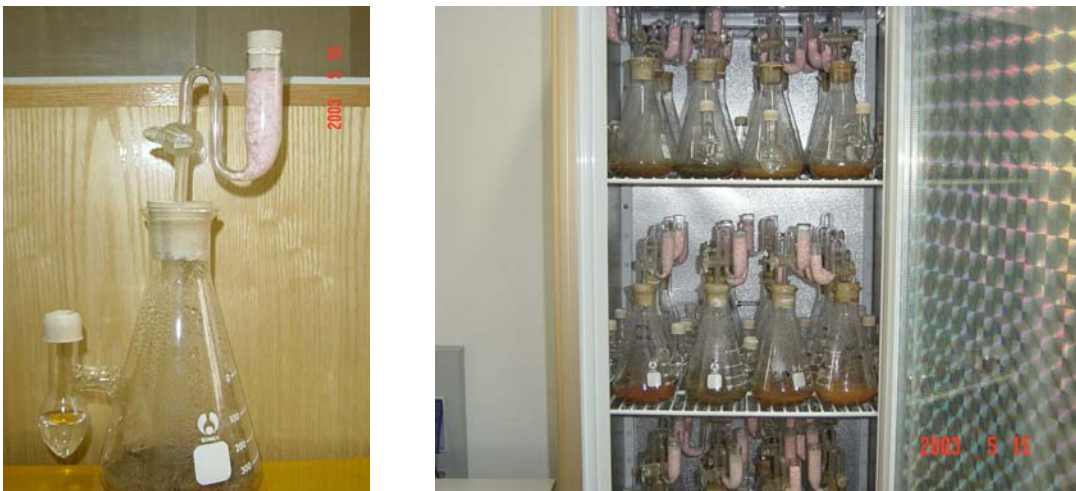
Figure 6. Incubation of soil samples to separate total soil carbon into fast, slow and passive pools for InTEC model parameters adjustments.
